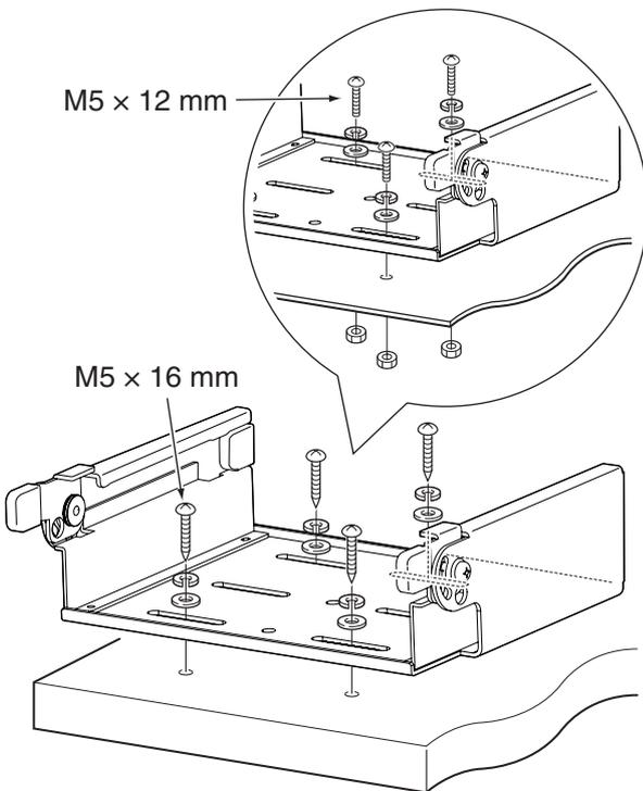
**⚠ WARNING!** Mount the mounting bracket to a surface that can support more than 10 kg (22 lb). The unit must be mounted on only a flat hard surface.
