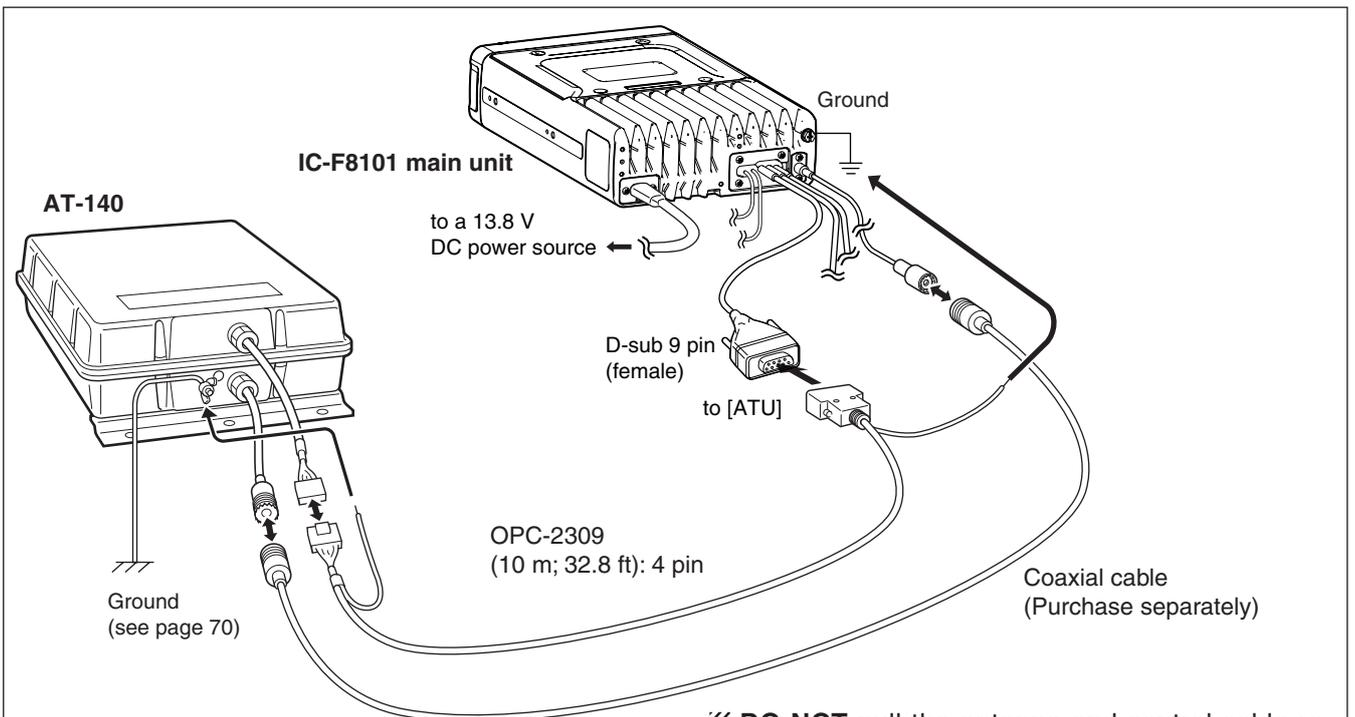
**DO NOT** pull the antenna and control cable receptacles. This may cause a cable disconnection (in the tuner unit), inside connector damage or a bad connection.
